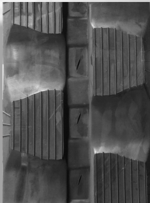
E-1 Mini Considered a block pattern but with tapered lugs. Commonly used on ride-on skid steers
